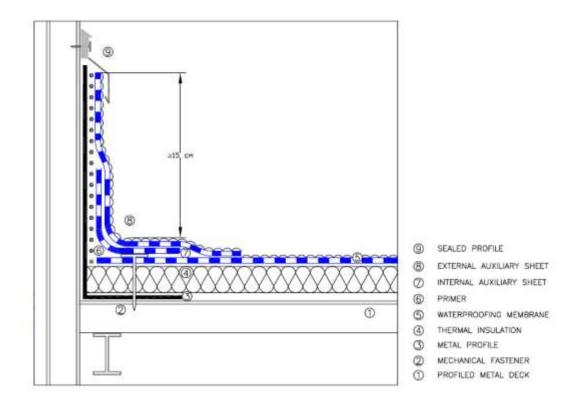
Fig. 3 Insertion with a vertical wall
