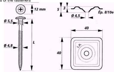
The length (L) of the fastener can be 65-75-80-90-100-110-120-130-140-150-160-180-200-220-240-260 mm. The fastener is made by Steel with an anticorrosion coat 2C.
