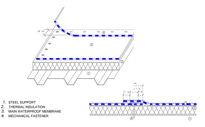
Fig. 2 Detail of a structural joint
